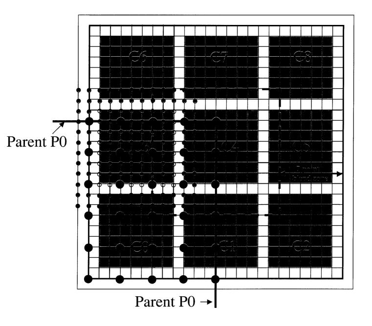
Figure 3. COAMPS child nest with 25 x 25 grid points and 3 x 3 domain decomposition. The heavy solid lines and larger solid circles represent the parent processor P0 as in Figure 2. The smaller open circles are the computational points and the closed circles are the two halo points of C3. The seven point blend zone is the area outside the dashed box.
