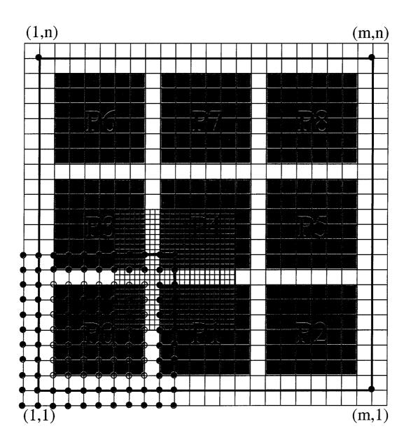
Figure 2. COAMPS parent nest domain similar to Figure 1, but in addition showing the overlap with a child nest. The open circles show the computational points and the closed circles show the two halo points of P0. The child nest is a  $25 \times 25$  grid point domain. The heavy solid lines through the center of the child domain represent the outer extent of the parent subdomain for P0 that intersect with the child domain, as shown in Figure 3.
