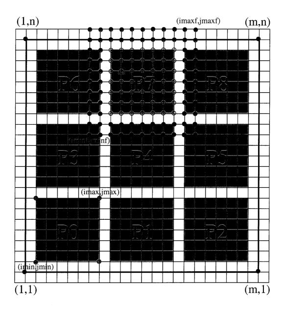
Figure 1. COAMPS single nest (m,n) 23 x 23 grid point domain for a 3 x 3 domain decomposition. The computational area of each subdomain in shaded. For subdomain 7 (P7) open circles indicate computational grid points and solid circles indicate the two halo points.
