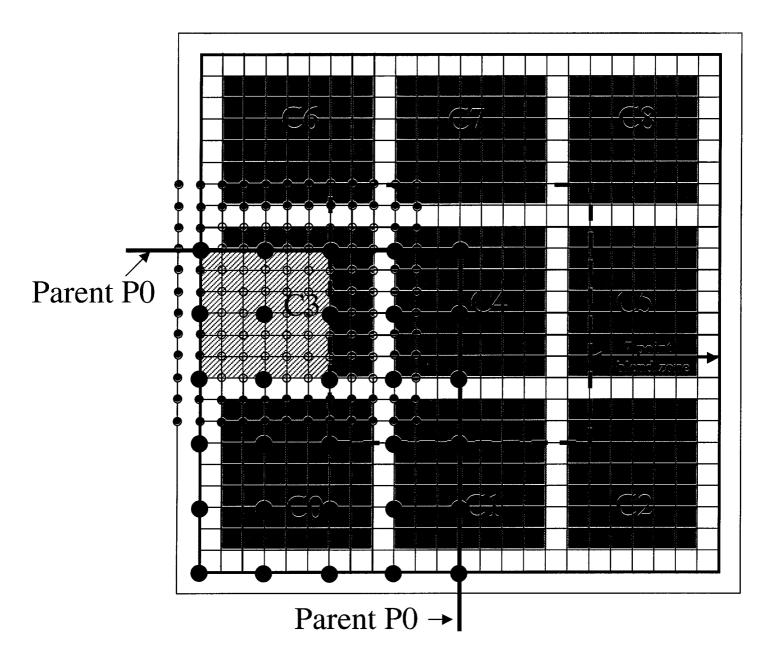
Figure 5. Sample COAMPS child nest and parent nest similar to Figure 3. The nine larger solid circles in the hatched region are the envelope of parent mass grid points that must be communicated from parent P0 to child C3 based upon the given seven point child blend zone. In this hatched region, mask values for parent and child nests are both equal to one.
