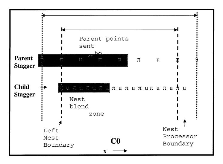
Figure 4. 1-D envelope structure for an Arakawa C-grid.
