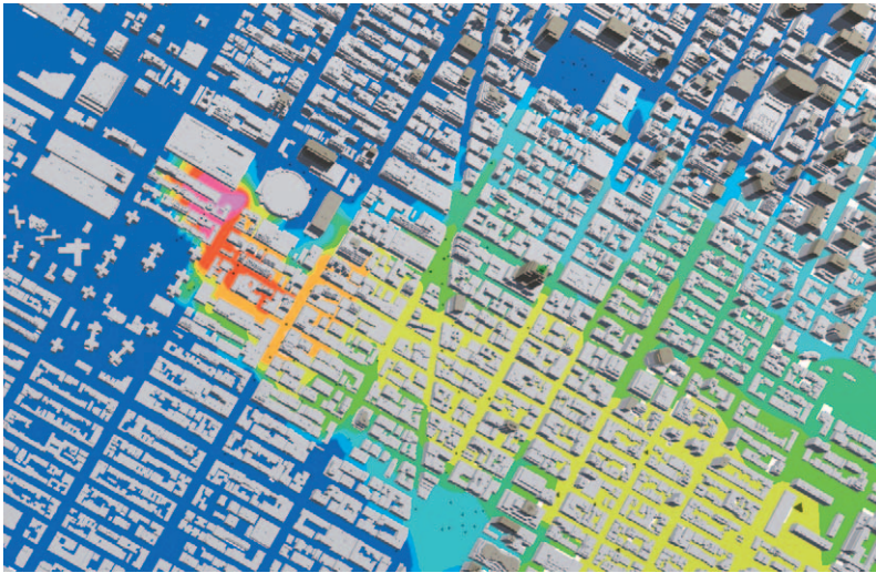
FIG. 19. CFD-Urban simulation of tracer gas dispersion for a point release near street level on the southwest side of MSG, for the west-northwest wind direction. This is one of the five source locations used during the MSG05 field experiment.
