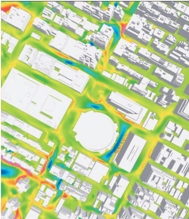
FIG. 13 (ABOVE). Simulations of vertical velocity w ( \text{m s}^{-1} ) at z = 2 m, by FLUENT-EPA for 10 Mar 2005 upstream wind inputs (flow from the northwest).
