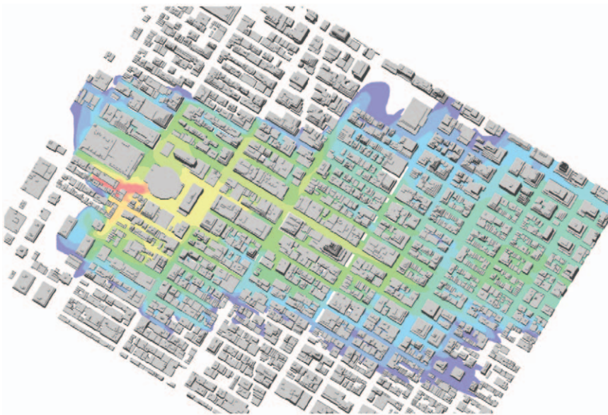
FIG. 20. FLACS simulation of tracer gas dispersion for a point release near street level on the southwest side of MSG for the west-northwest wind direction. This is one of the five source locations used during the MSG05 field experiment. The figure is for 900 s after the release was initiated.
