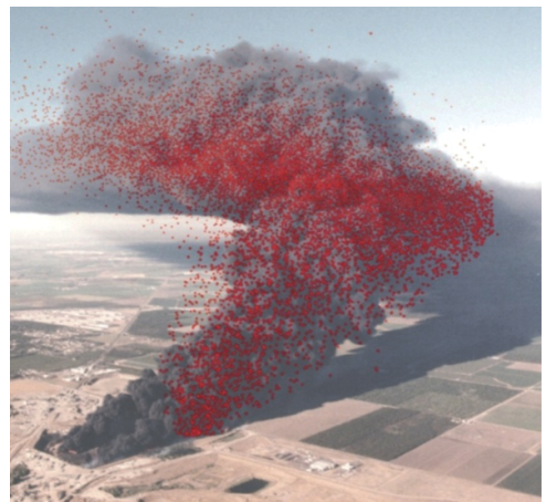
Smoke plume photograph with NARAC-simulated smoke particles in red for a tire dump fire. (Photo courtesy of Tracy Press)
