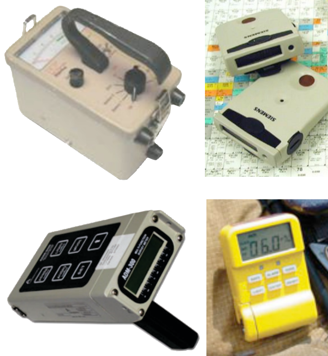
Figure 42. Example high-range instruments for dose-rate assessment. (These are pictures of common radiation detection instruments as examples. The use of these images does not represent an endorsement by the authors.)
