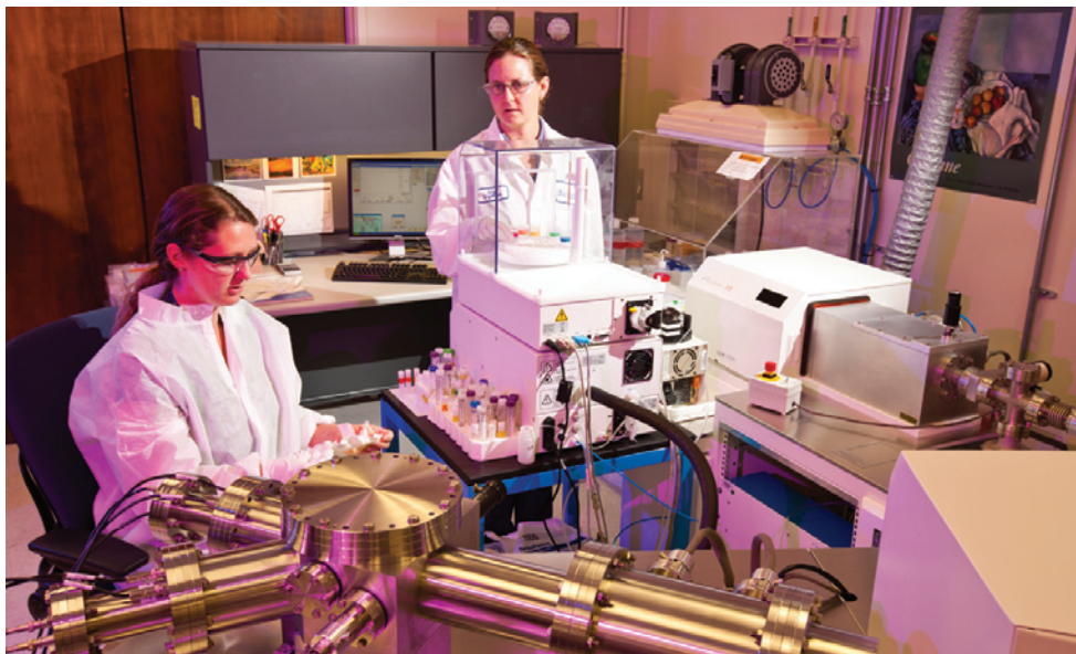
Livermore chemists Rachel Lindvall (left) and Amy Gaffney (right) analyzed Japan air particulate samples for uranium and plutonium isotopic composition with Nu Plasma HR™, a multicollector, inductively coupled plasma mass spectrometer.
